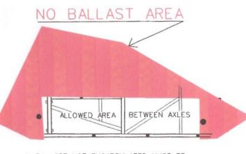
ANY BALLAST NOT ENCAPSULATED MUST BE PAINTED WHITE AND BE IDENTIFIABLE BY CAR NUMBER. ALL BALLAST MUST BE APPROVED BY TECH OFFICIALS.
