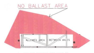
ANY BALLAST NOT ENCAPSULATED MUST BE PAINTED WHITE AND BE IDENTIFIABLE BY CAR NUMBER. ALL BALLAST MUST BE APPROVED BY TECH OFFICIALS.
